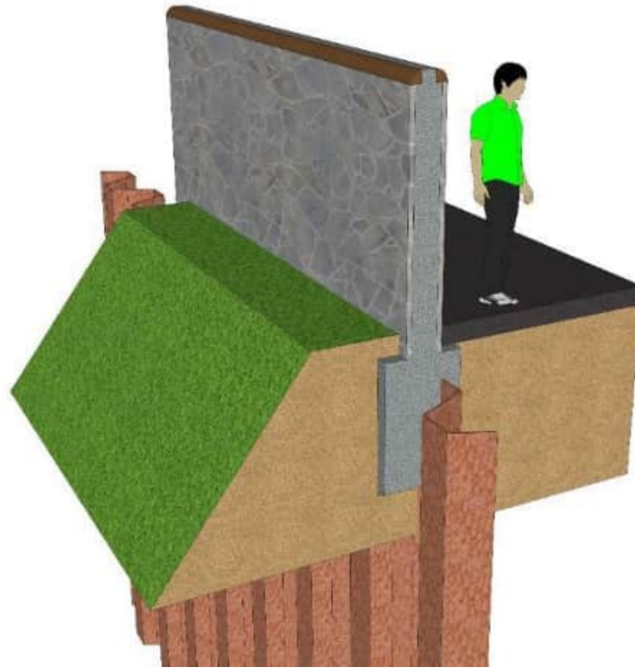
Figure 6: Schematic of Sheet Pile Wall with reinforced concrete stem (at top of riverbank)
