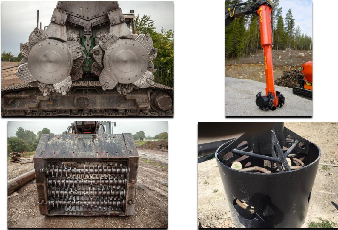
Figure 5 Range of different mixing heads for soil mixing. Photo courtesy of Deep Soil Mixing
