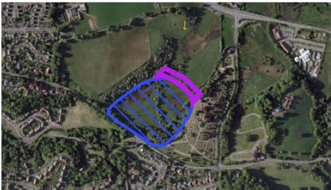
Figure 3-31: Alignment of embankments (purple) and extent of (emergency) flood storage area (blue hatch) (Yellow arrow indicates position and direction of photo)
